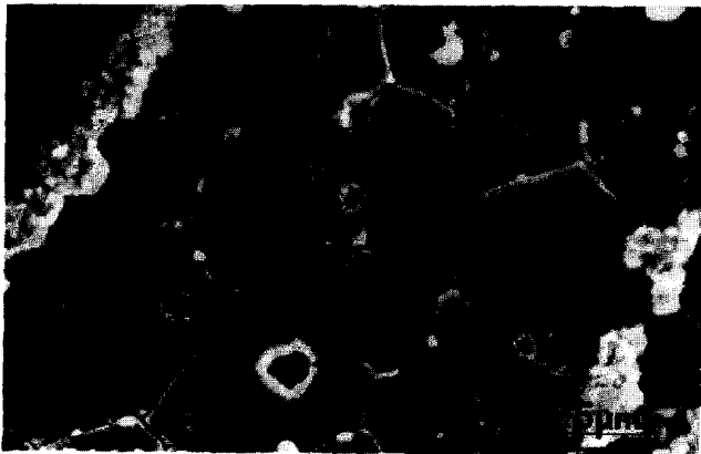
Fig. 9. Backscattered electron image of a thermally etched VP1 sample sintered at 1050°C for 1 h indicating single spinel particles at grain boundaries and spherical pores and spinel particles within ZnO grains. Z = ZnO, S = Spinel and Pr = Pore.
